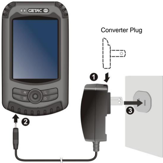
3. The multi-functional indicator glows amber when charging is in progress. Do not disconnect your Pocket PC from AC power until the battery is fully charged. This will take a couple of hours.
