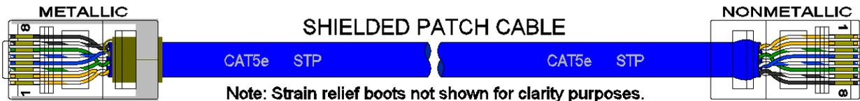
In the event all Cat5e patch cable distances are small (i.e. All Ethernet devices are located the same local cabinet and/or referenced to the same earth ground), it is permissible to use fully shielded cables terminated to chassis ground at both ends in systems void of low level analog signals.
