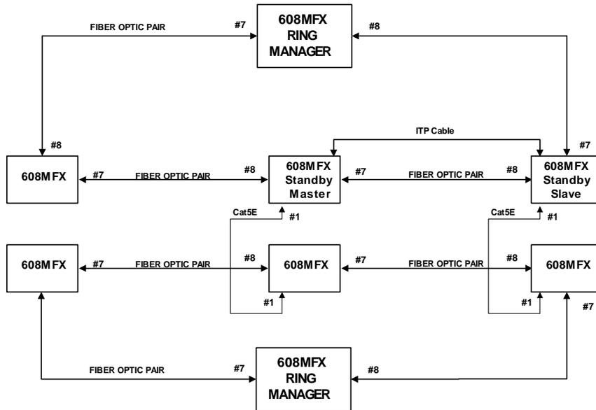
**608MFX Network Segment Redundancy
