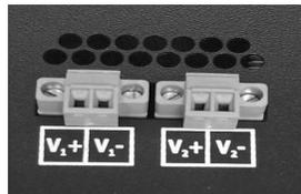
Unscrew & Remove the DC Voltage Input Plug(s) from the side header
