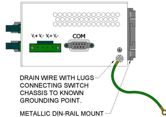
The use of shielded cables between devices is not required for most N-Tron devices (please consult the user manuals for specific details). If the use of shielded cables is required, it is generally recommended to only connect the shield at one end to prevent ground loops and interfere with low level signals (i.e. thermocouples, RTD, etc.). Cat5e cables manufactured to EIA-568A or 568B specifications are required for use with N-Tron Switches.
