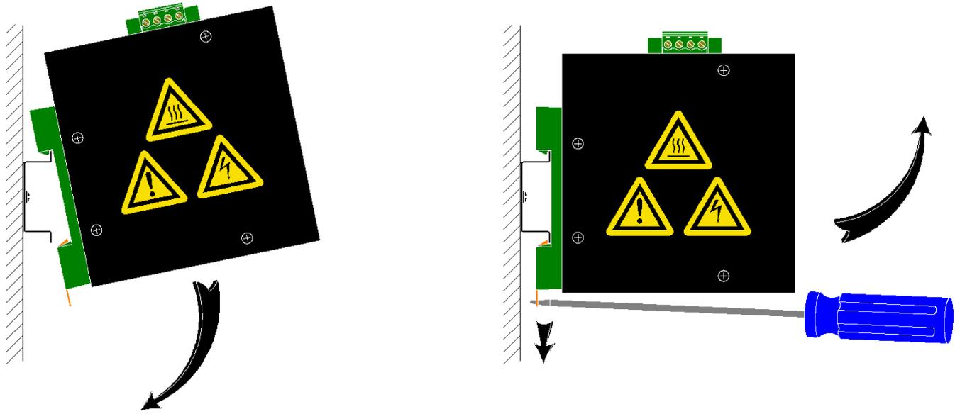
To install the unit to 35mm industrial DIN-Rail, place the top edge of the included mounting bracket on the back of the unit against the DIN-Rail at a 15° angle as shown. Rotate the bottom of the unit to the back (away from you) until it snaps into place.
