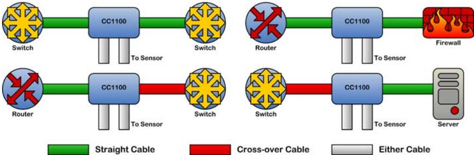
**Note:** This cable guide is for 100MB operation only and is to ensure that the LAN devices can still communicate even if power to the TAP fails. It is not necessary for 1000MB operation as Auto-MDIX is used. Most equipment vendors follow the above standard MDI or MDIX configurations, however some vendors may not. To ensure proper connectivity, always verify link at the network devices with the TAP power off. If there is no link try changing one of the cables from Straight-thru to Cross-over.
