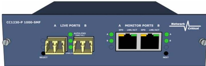
The CC1230 is part of the new generation of TAP products from Network Critical; it is a fully featured, fully configurable tapping solution for singlemode fiber network links, with support for up to 2 gigabit network tools.
